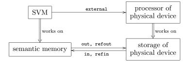
Figure 3.2: Interaction of the SVM with the physical device
